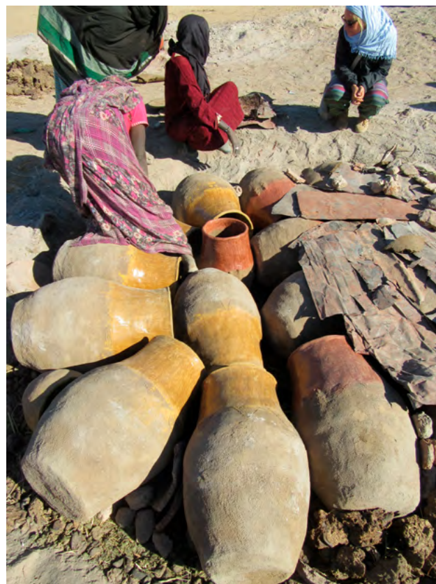
Figure 19 ▲◀ Pottery kilns in Jabarūna village in the form of a pit with metal shreds and plates at the top as isolation to protect vessels from the flames and different stages of the firing preparation. Photos by B. Franczyk.
